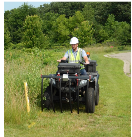
Mobile leak survey in rural road right-of-way
