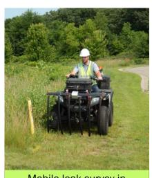
Mobile leak survey in rural road right-of-way
